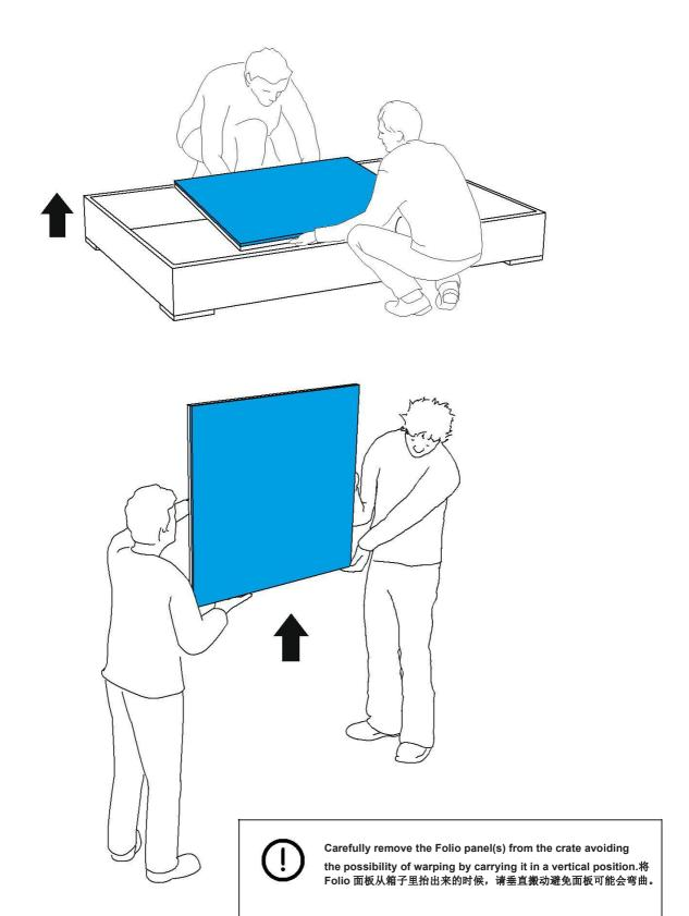
Carry the panel always keeping it in the same vertical position, avoiding hitting, pulling or damaging the electrical cables. Avoid contact of Folio panels with liquids.搬动面板请一直保持同一垂直方向,避免碰撞 拉伸损坏电力电缆,避免面板接触到液体。
