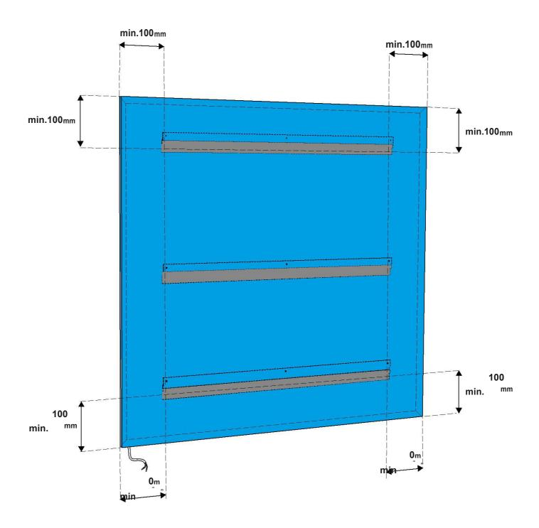
The figure shows the exact position of the brackets for mounting. 图中显示安装支架的正确位置。 The brackets shown are fixed to the
